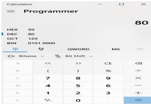
**Figure 8: Calculator to convert Decimal to Hexadecimal**
